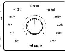
the *FBK* knob acts like a standard feedback control. turn this knob up to get more ascending/descending pitch bends. the *PIT* knob determines the pitch interval the pitch shifter is tuned to (see PIT note). the *DET* knob determines how much pitch shifting is happening. turned CCW there is no pitch shifting. increasing CW will increase the amount of pitch shifting.
