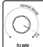
labeled **FRZ** short for freeze. this knob controls the amount of non additive feedback. when turned fully CW, the signal is frozen, meaning incoming audio is muted and the sound in the delay line is repeated infinitely.
