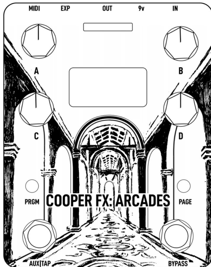
Knobs A, B, C, and D control the parameter that it is associated with, as dictated by the text on the screen.
